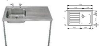
Sink bowl with drainer suitable for mouting on 1000mm wide and 1200mm wide sink base cabinets, Stainless Steel support legs or Wall mounted brackets. Bowl size 400mm x 400mm x 200mm deep. Standard bowls supplied with 200mm centre tap holes. Sink top with 50mm rear upstand available if required at additional cost.
