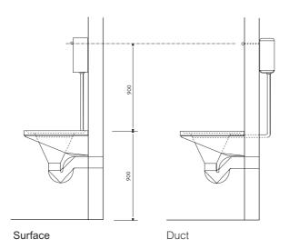
A DUH hospital disposal unit manufactured from 1.2mm thick, grade 1.4301 (304) stainless steel with a satin polish finish. The top is turned down on all four edges and incorporates a wet area recess. Fitted with a sluice hopper at one end which can be supplied with either top inlet or back inlet. The hopper has a 110mm dia. outlet which can accept a P or S trap, available as an extra.
